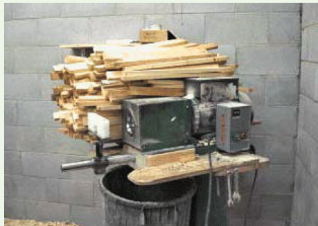
EQUIPMENT SUCH AS THIS SURVEY STAKE POINTER IS USED AS BOTH AN EDUCATIONAL AND PRODUCTION TOOL AT THE CENTRE
